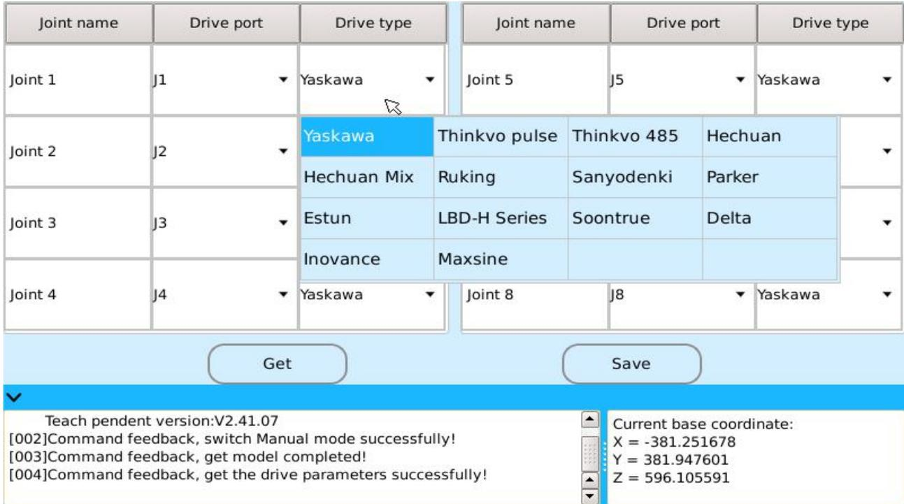
Figure 3.3\_2 Driver Configuration Interface
