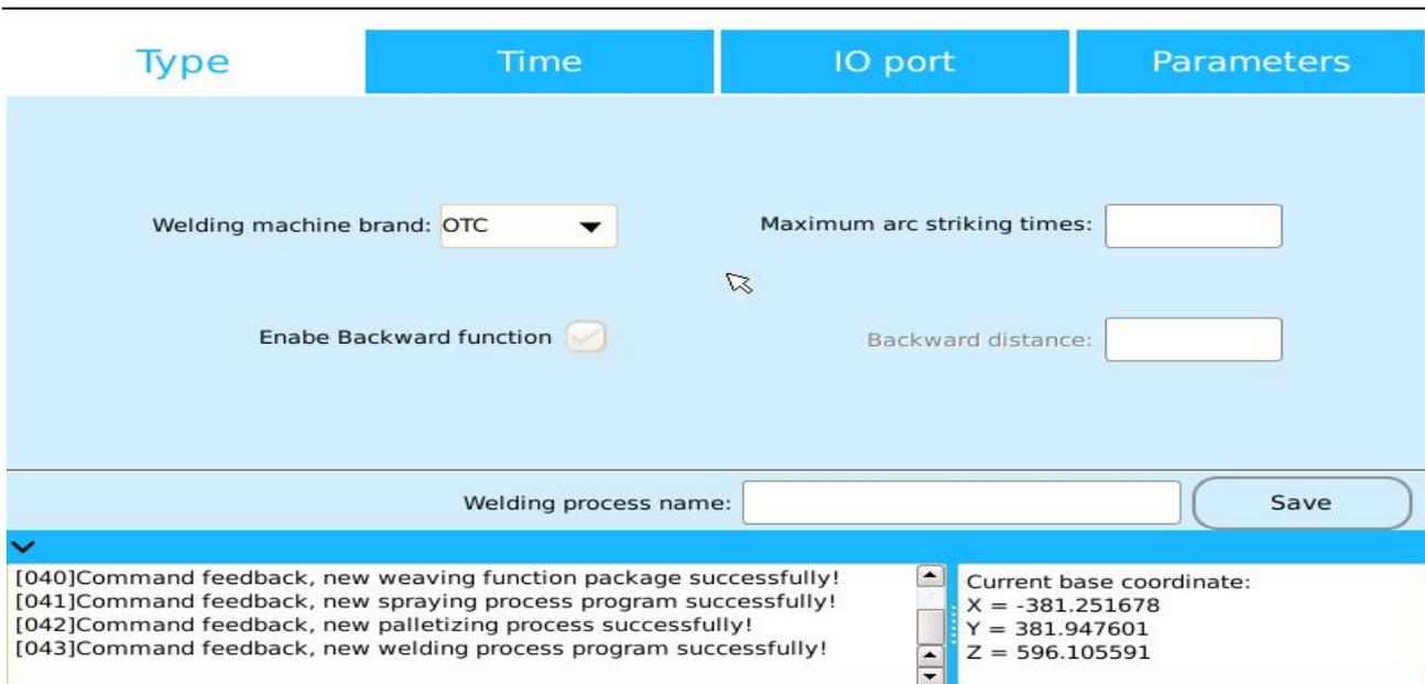
Figure 8.14 welding procedure Creation Interface
