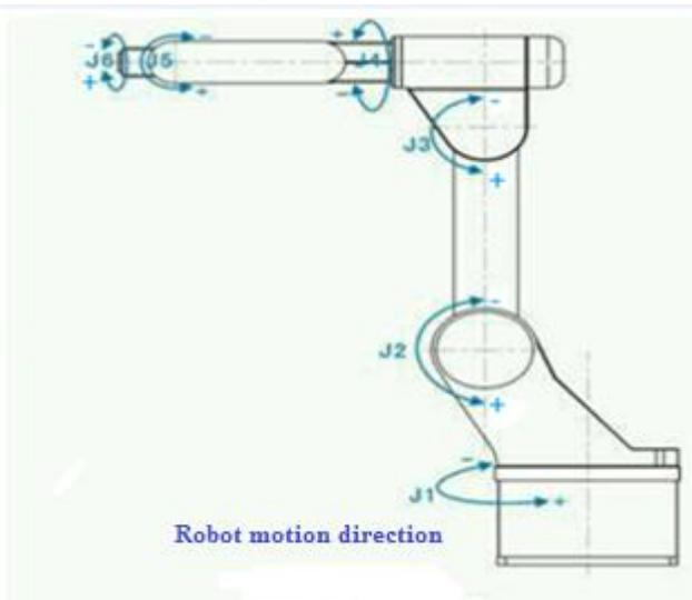
**The direction of motion of each articulation identified when a person stands at the rear of the robot body**
