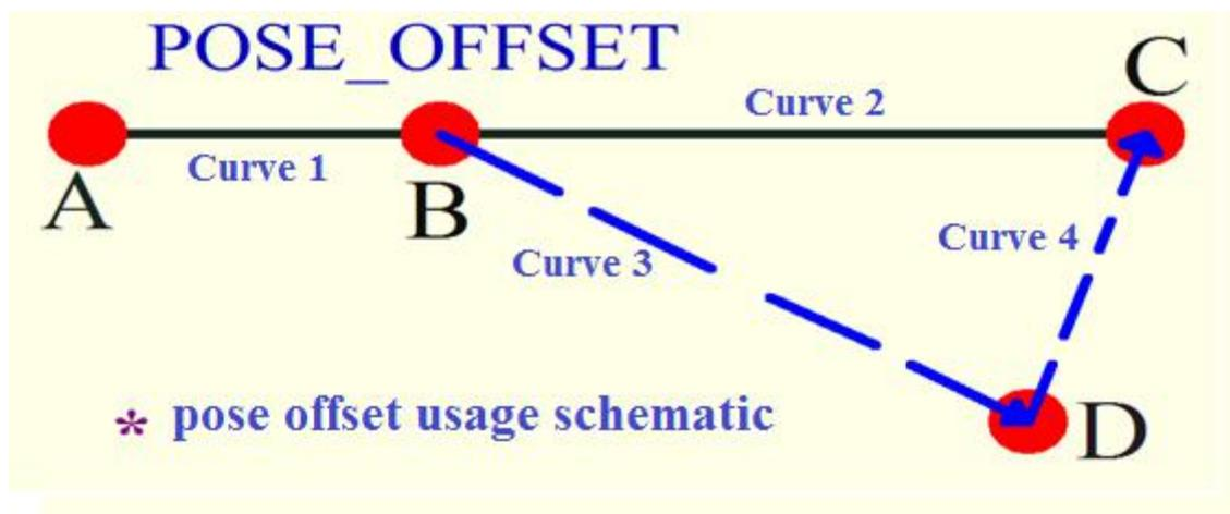
Curve 1:A-B;Curve2: B—C;When the "POSE\_OFFSET" task type is not used, the running track of the program is "A—B—C"; When the "POSE\_OFFSET" task type is used at the curve 1(i. e. the B-point position), the "point"s running track offsets from the current point "B" to the "D" point position, then runs to the "C" point position, that is, after the "POSE\_OFFSET" task type is used, The program's running track is turned into a "A-B-D-C".
