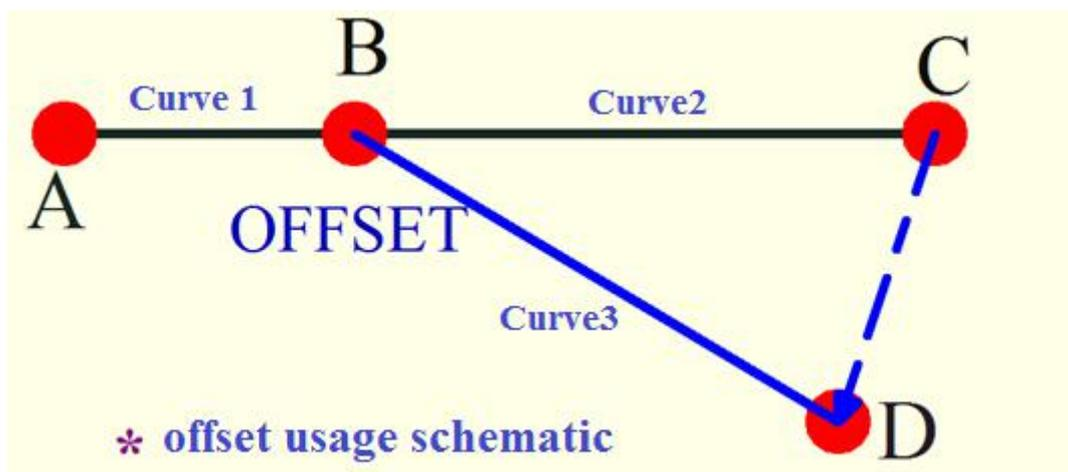
Curve 1:A-B;Curve2: B—C;In the absence of the “OFFSET” task type, the complete trajectory of the curve is “A-B-C”; After using the "OFFSET" task type after curve 1(i. e., at the point "B"), the terminal point "C" of the original curve 2 will be OFFSET to the position of "D", so the curve trajectory of the program after using the "OFFSET" task type becomes "A--B--D".
