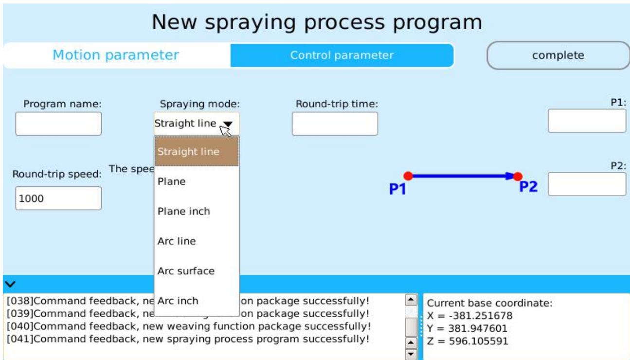
Figure 8.2 Spraying Procedure Creation Interface
