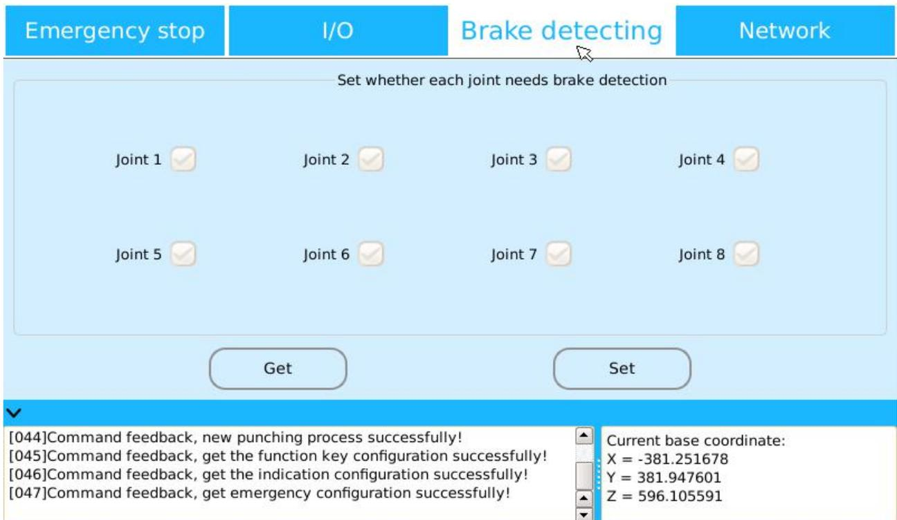
Figure 9.9 configuration of “brake anomaly detection”
