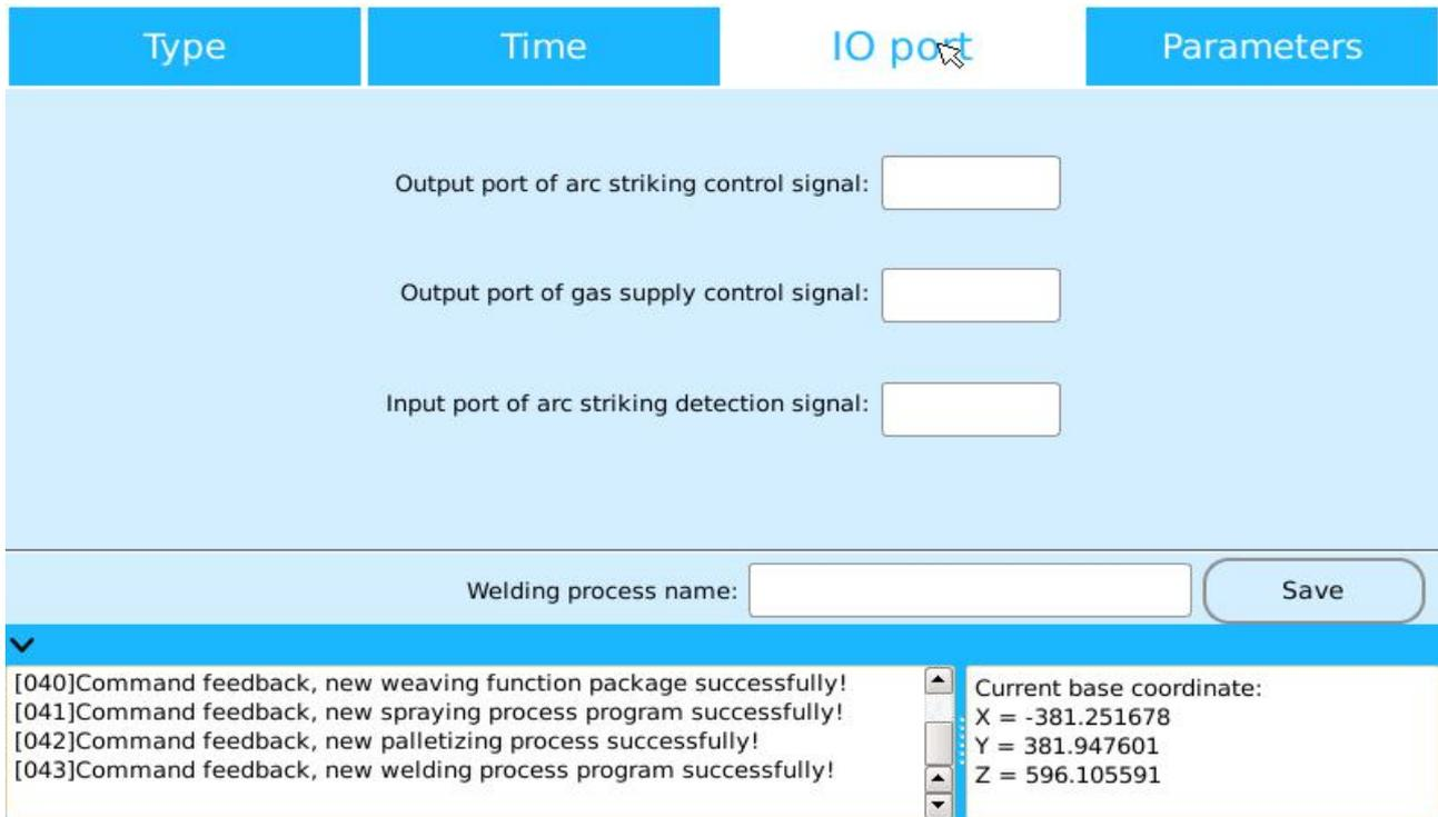
Figure 8.15 “welding procedure” IO port settings interface
