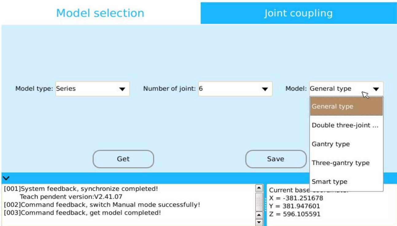
Figure 3.2 machine model setting interface
