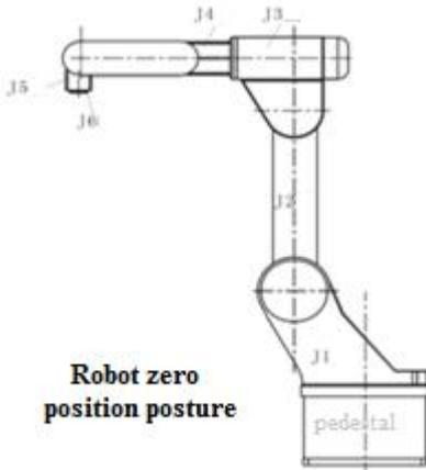
As shown in the left figure, move each joint of the mechanical arm body to each position in the left figure. In the "machine parameters" setting interface (as shown in figure 3.4), click the button "set zero-bit angle" -- "query" to complete the setting of "zero-bit angle" of the system.
