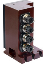
Four power heads on the Y axis side
